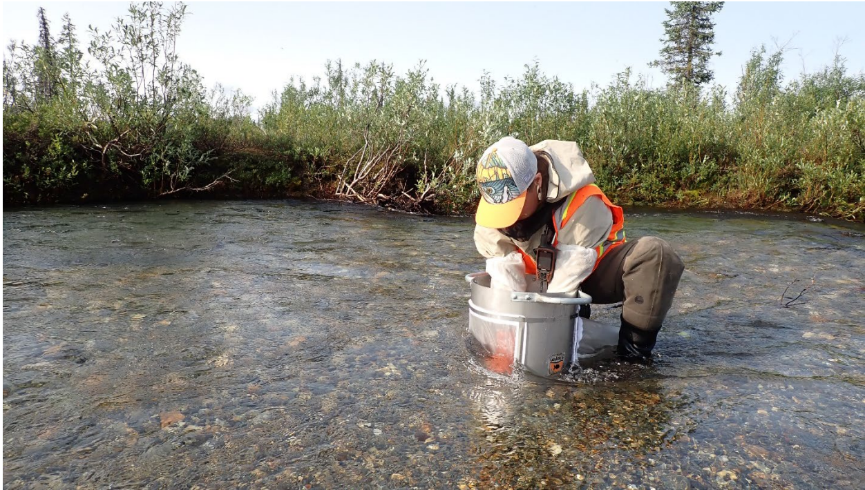
Figure 5. Collecting invertebrate samples using a Hess sampler on Lower Subarctic Creek.
