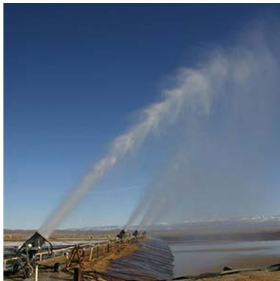
Figure 3-5: Typical Tailings Facility Air Blast Evaporators
