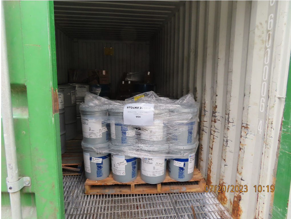
Photo 4. The 920 warehouse storage container with secondary containment.
