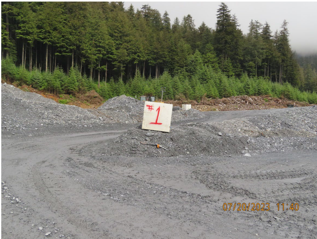
Photo 7. Waste rock storage area Site 23. Class 1 waste rock is separately staged from class 2/3 waste rock.
