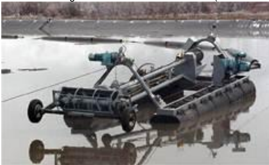
Figure 16: Crisafulli “Flump” Dredge with Liner Protection System
