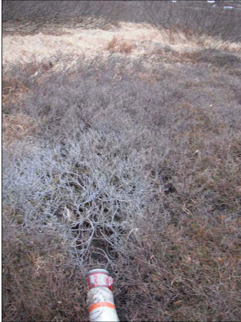
Figure 4. End of sump pit discharge line. Ground is temporarily discolored from drill water that was previously discharged. Water absorbed well in immediate area and with no run-off visible.
