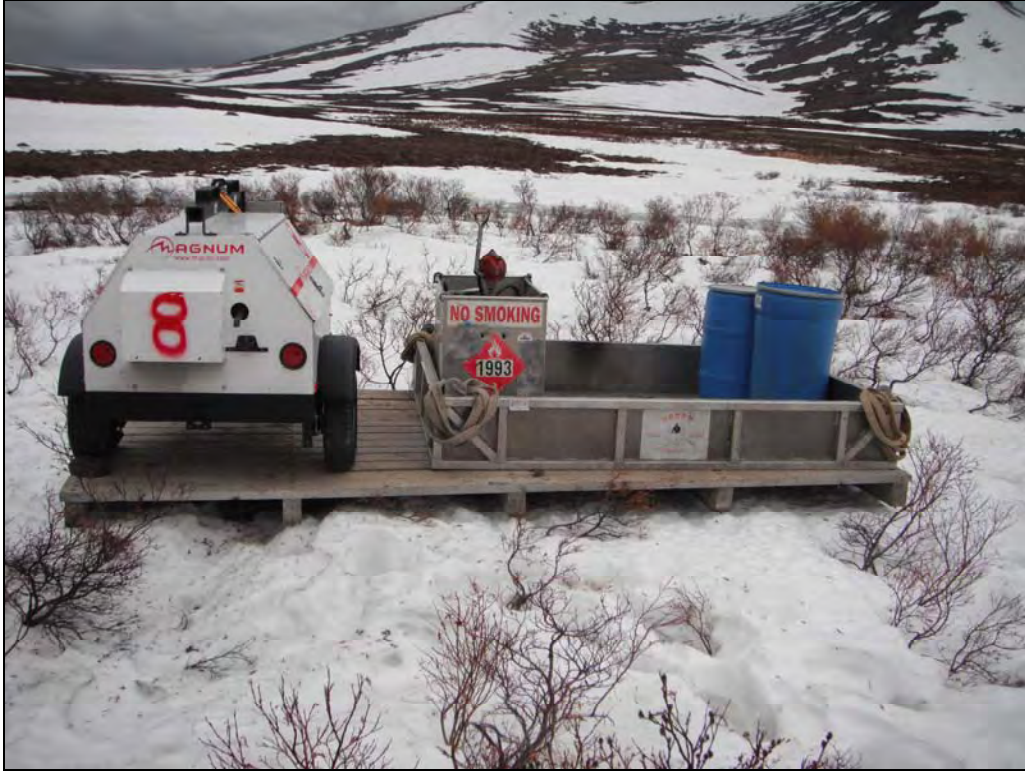
Figure 15. Fuel and generator used for water pump.
