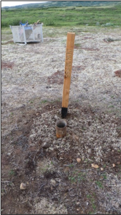
DDH12555 marker and drillhole pipe. Reclamation kit is in the background.
