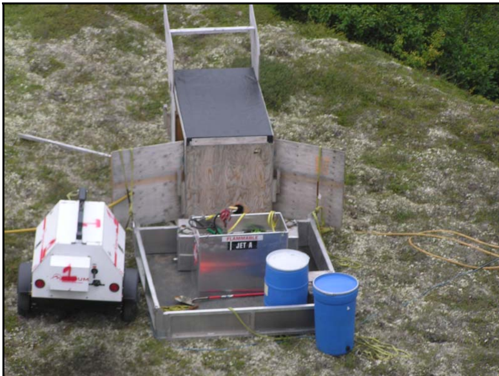
Figure 4: Water pump for Drill Rig # 8.
