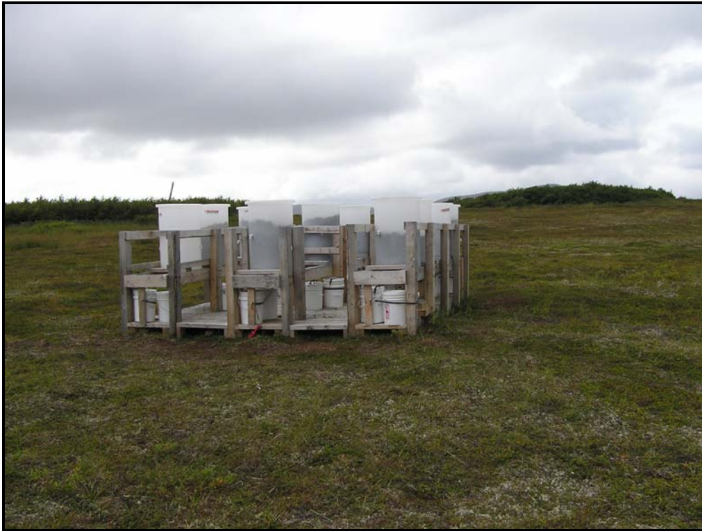
Figure 34: Geochemical barrel testing station.
