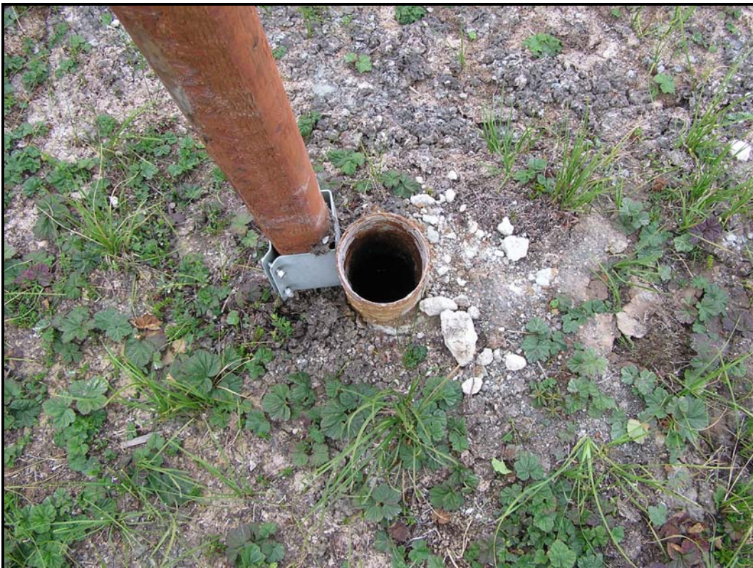
Figure 31: Open casing for DDH # 8405; unable to determine if hole had been plugged.
