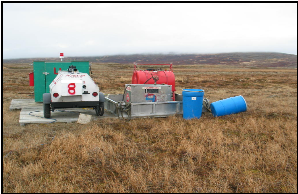
Figure #4: Drill #4. Water pump. Fuel is in containment, with spill kit and scrubber barrel.
