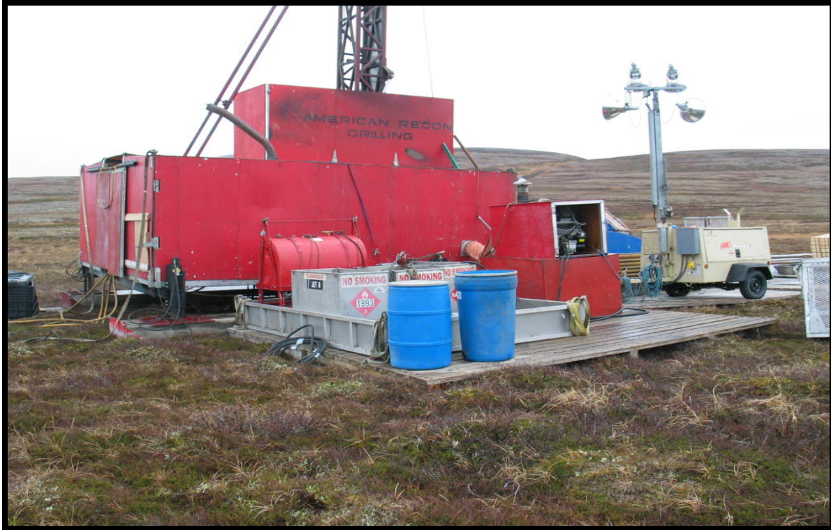
Figure 1: Drill #4 on DDH 9473. Note fuel containment, spill barrel and oil scrubber, tundra pads.
