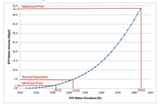
Figure 2: RTP Volume-Elevation Curve
