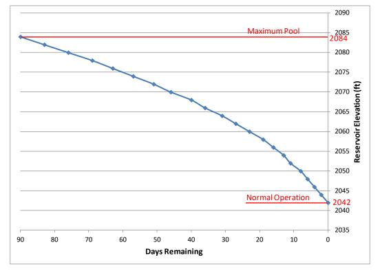
Figure 3: Drawdown Curve for 300 gpm Discharge from RTP
