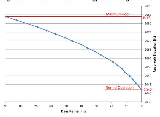
Figure 3 Drawdown curve for 300 gpm discharge from RTP
