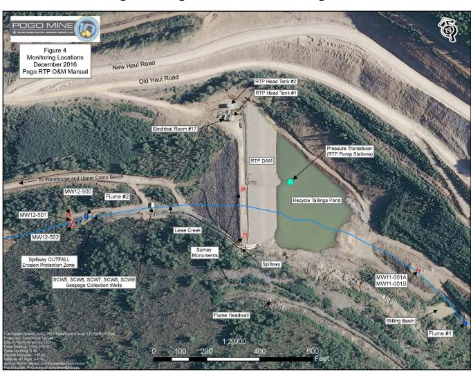
**Figure 4 Pogo RTP Dam monitoring locations**
