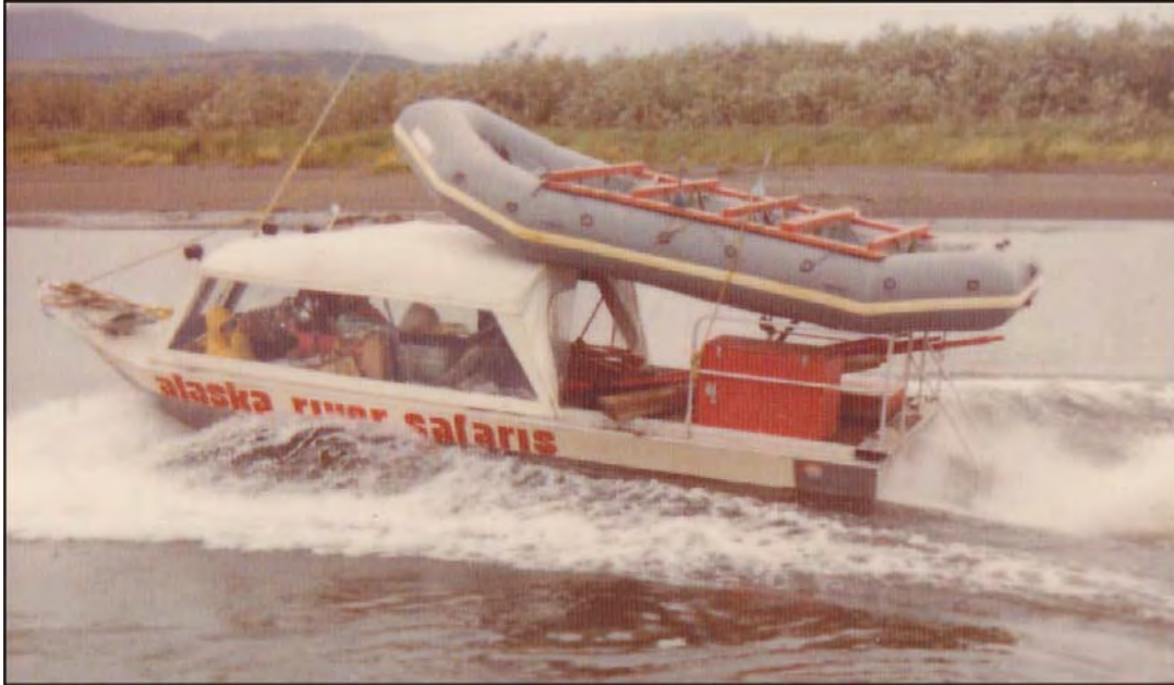
Figure 10. Hauling a raft up the Goodnews River on a jet boat in the late 1970s. The jet boat is a 25-foot Duckworth with a 454 cubic inch Chevy engine and a 3-stage Hamilton inboard jet unit.
