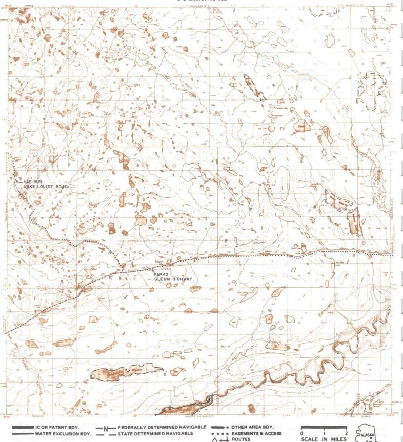
FAP 42 Omnibus Road easement extending 150 feet on each side of the centerline of the Glenn Highway.
