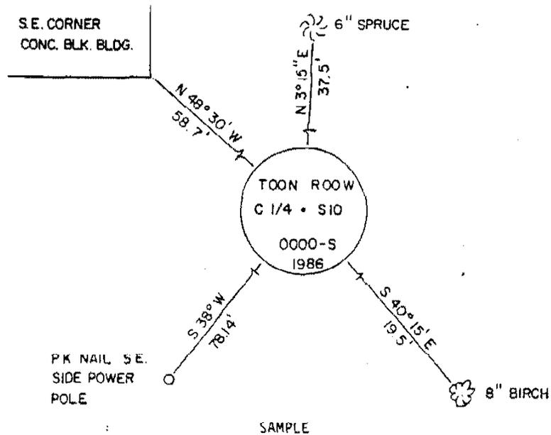
5. PREPARE A SKETCH SHOWING THE MONUMENTS USED AND MEASUREMENTS MADE TO DETERMINE THE POSITION OF THE MONUMENT BEING ESTABLISHED:
