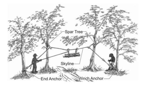
Figure 6.22 – Cable Winch Rigging System
