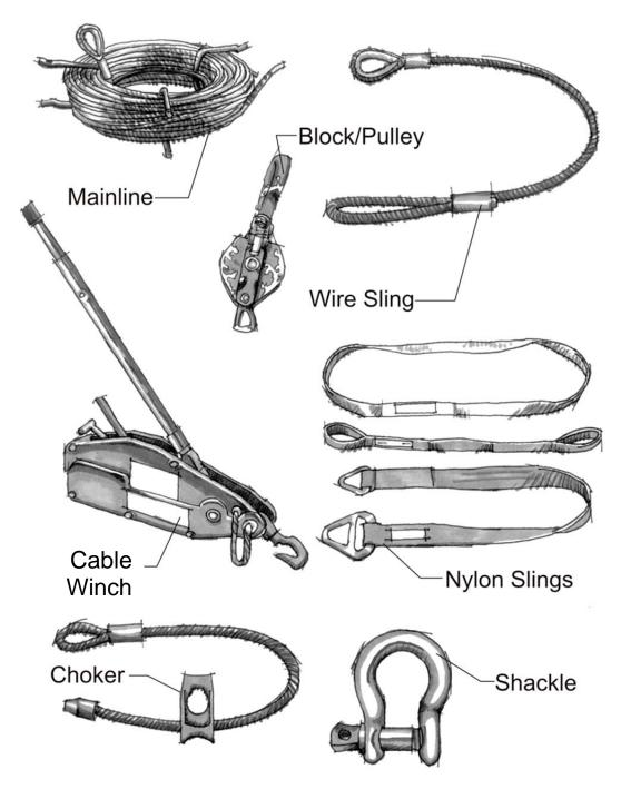
Figure 6.27 – Cable Winch and Common Accessories
