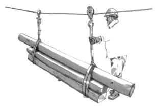
Figure 6.24 – Logs on mainline with slings and pulleys
