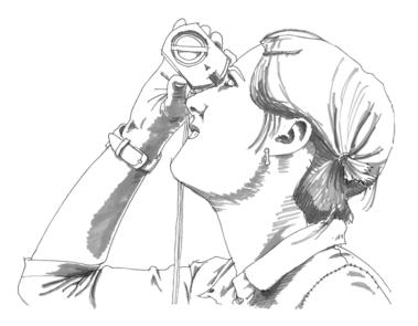
**Figure 6.21 – Holding a Clinometer**
