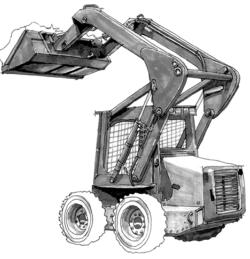
Figure 6.36 – Skid-Steer Loader
