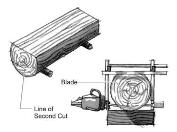
Figure 6.29 – Alaskan Saw Mill: 2<sup>nd</sup> Cut
