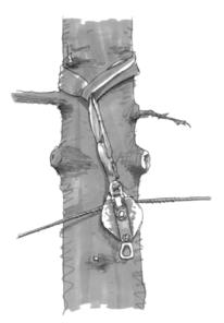
Figure 6.23 – Nylon sling around spar tree with pulley and mainline
