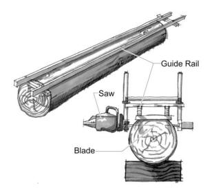
Figure 6.28 – Alaskan Saw Mill: 1<sup>st</sup> Cut
