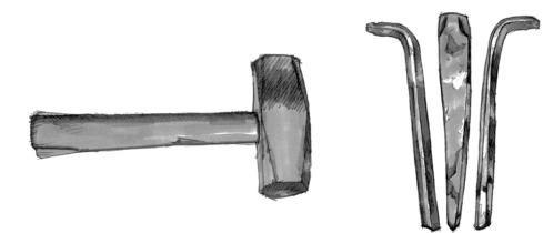
**Figure 6.32 - A Plug and Feather Hand Splitting Tool Set**: 8lb Double Jack and Two Feathers (Shims) with Plug (Wedge)
